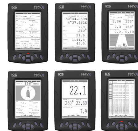
NMEA repeater and data logger views
