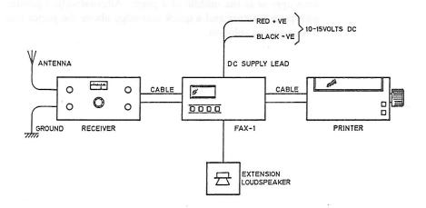
CAUTION: When connecting or disconnecting leads, ensure that the equipment at both ends of the cable is switched OFF.
