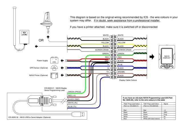
Programming Cable wiring for NAV6 displays with software earlier than Version 1.5 using the a V2 or eNAVTEX antenna replacement (black box)
